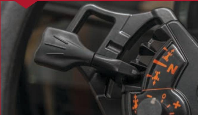
All Global Series tractors come with a clutch control button on the gear shift for simple and clutch pedal-free gear shifting. To change gears in Global Series tractors, press and hold the clutch control button, shift to the desired gear, and let off the clutch control button.
